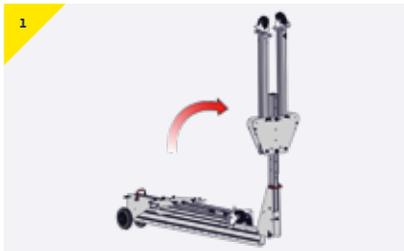
Rotate upper A-Frame to a vertical position.
