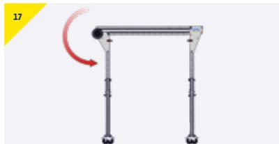
**If fitted, ensure castor brakes applied before lifting a load.**
