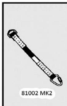
A 0.5m lanyard to EN354 fitted with a 'D' ring and screwed triangular link designed to extend a harness fall arrest attachment point. It must ONLY be used with a retractable type fall arrestor (EN360) incorporating an automatic tensioning spring. Connect the screwed triangular link directly to your harness fall arrest 'D' ring. Connect the
