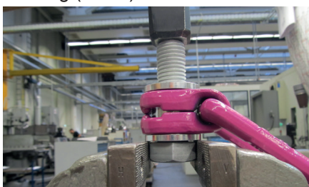
Pic. 8: Dismantling position of the VLBG-PLUS
