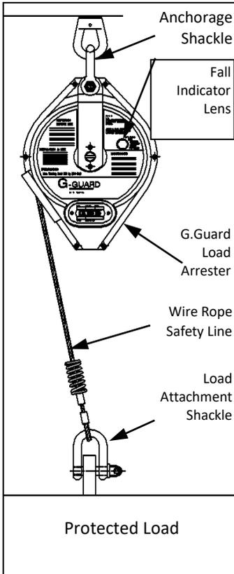
In the event of a fall, rope is pulled out of the unit at an accelerating rate. On reaching the activation speed the braking mechanism will engage. The energy of the fall is dissipated and the load brought to a halt. There should be adequate clearance below the protected load to safely stop a fall.
